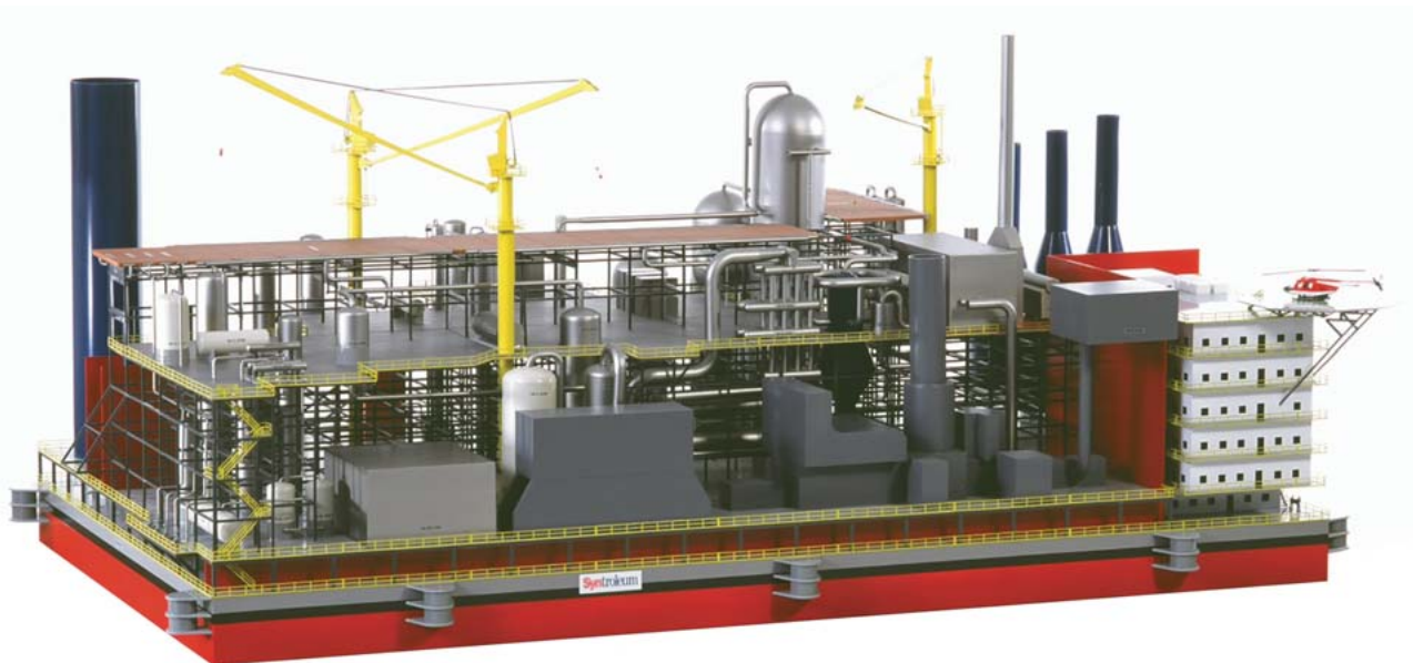
Figure 1. The Syntroleum GTL Barge, whose commercial design provides the basis for the GTL FPSO currently being designed, measures 250 ft (76 m) by 450 ft (137 m) by 11 ft (3 m) draft. Grupo Dragados S.A. of Spain is ready to help finance and build the barge. Syntroleum hopes to have a project ready for GTL production by 2009. (Image courtesy of Syntroleum)
