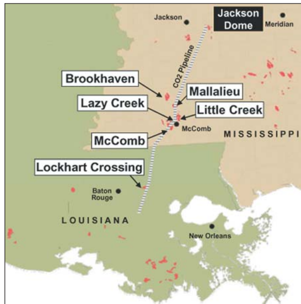
Figure 1. Two primary operating areas include Eastern and Western Mississippi, with the 183-mile (295-km) CO 2 pipeline starting at Jackson Dome, extending to White Castle, La. (Image courtesy of Denbury Resources Inc.)
